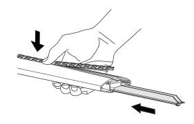
Install the rubber molding by pressing downward and cutting it to fit the ends.
