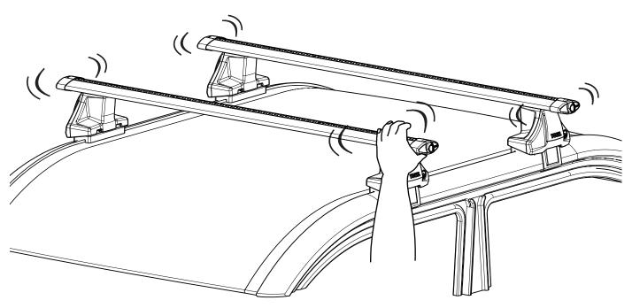
Push and pull in all directions to make sure the roof racks are installed firmly.
