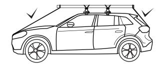
Do not drive faster than 50Mph (80 km/h) with long loads.
