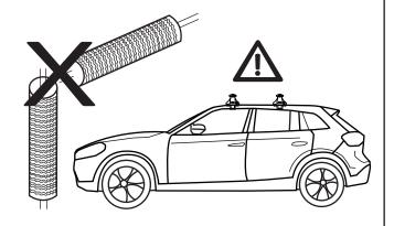
Check the height of the vehicle when roof racks and attachments are installed before driving under tunnels or parking structures with low bridges.
