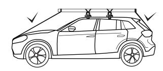
Do not drive faster than **50Mph (80 km/h )** with long loads.
