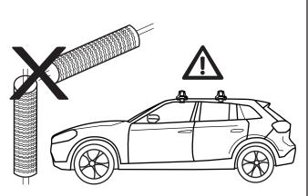
Check the height of the vehicle when roof racks and attachments are installed before driving under tunnels or parking structures with low bridges. When using an automatic car wash, roof racks and attachments must be removed.
