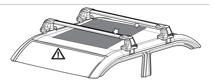
Precaution must be taken as the sunroof may interfere with roof racks or mounting gear.
